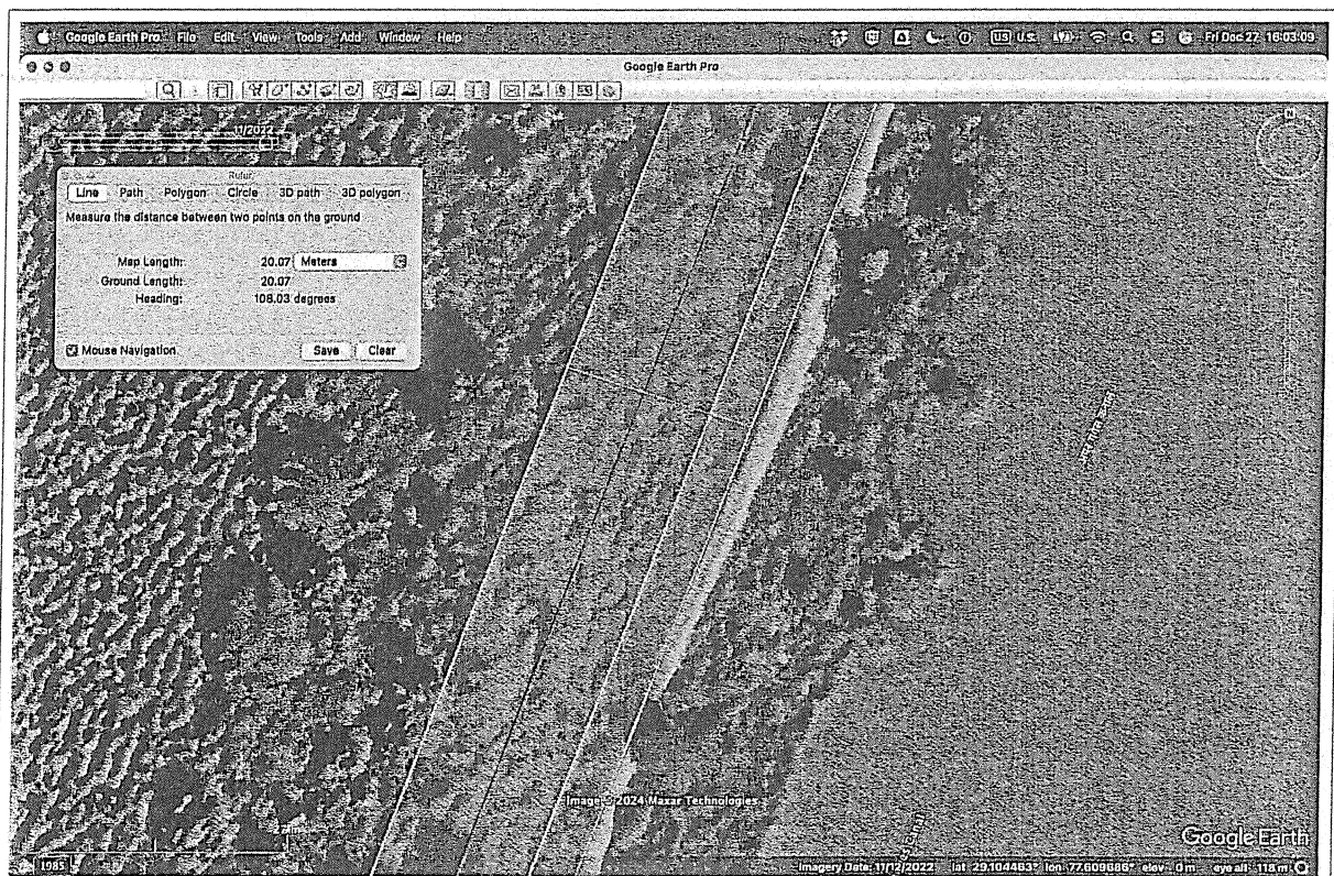
Fig 2. The width of the strip proposed to be cleared of vegetation is 20 meters. This includes the central carriageway depicted in blue, and surrounding strips depicted in yellow colour. The coordinates of the site, and the date of satellite imagery are depicted at the bottom of the image.
